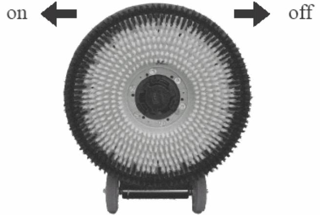
To install a brush or pad driver, leave the handle in the upright position and tip the machine backwards. The brush and pad driver both attach in the same manner. Align the 3 cut-outs on the clutch plate with the 3 cut-outs on the drive hub. Push the brush/pad driver on to the drive hub and turn it counter clockwise to lock it in position.
