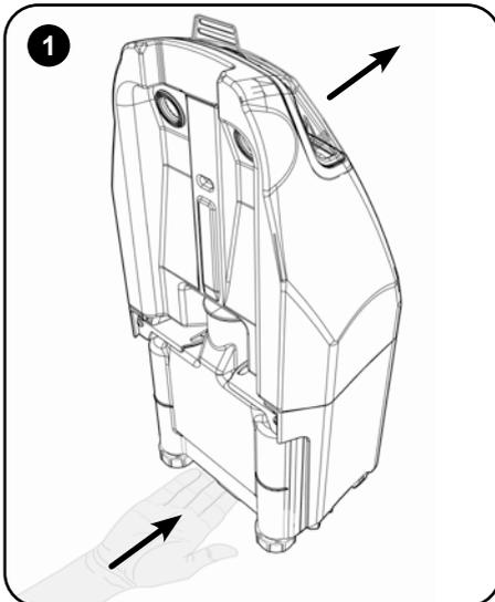
After lifting onto a suitable work surface, tilt the tank assembly slightly forward and slide your hand under the tank.
