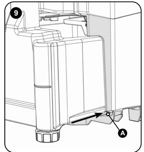
Pour in the chemical (follow chemical manufactures dilution rates). Only fill the tank to the MAX fill line with clean water using a tap, hose or suitable water container. DO NOT OVER FILL. Slide the tank back into the main tank body, make sure the front of the clean water tank is lifted to enter the recess (A). Push the tank all the way in until you hear it click, make sure it is securely fitted before fitting the tank assembly back on the machine.
