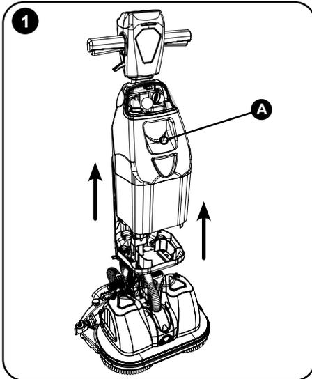
Remove the tank assembly from the front of the machine. Using the inset handle on the front of the tank assembly (A), lift the tank assembly up towards the main handle.
