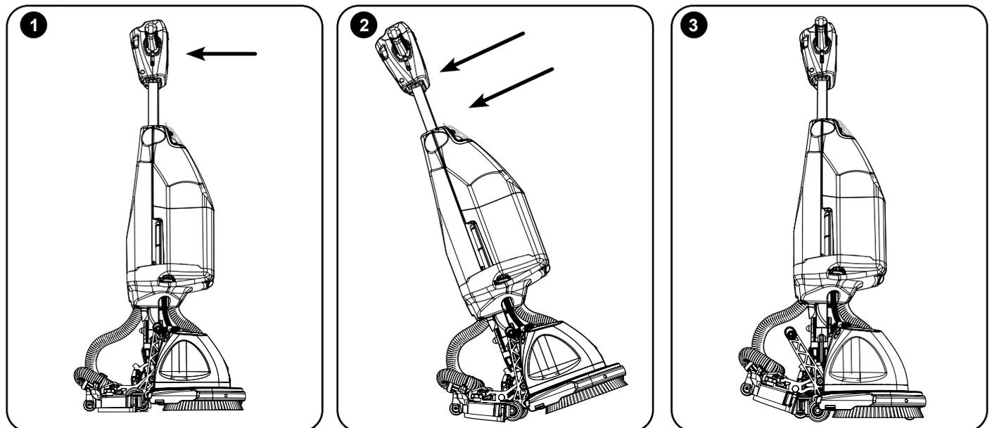
To put the machine into storage mode start with the handle locked in the upright position and the floor-tool down (1), pull the handle backwards until the floor-tool moves up and the transport wheels click out into position the front support wheel is deployed (2). Rest the machine back onto the transport wheels (3) (no button or lever action is required). Note: Do not let go of the handle.
