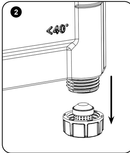
Remove the clean water outlets from the clean water tank.
