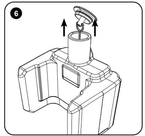
Remove the clean water tank from the main body of the tank holder (4&5). To fill remove the rubber stop from the filling neck.
