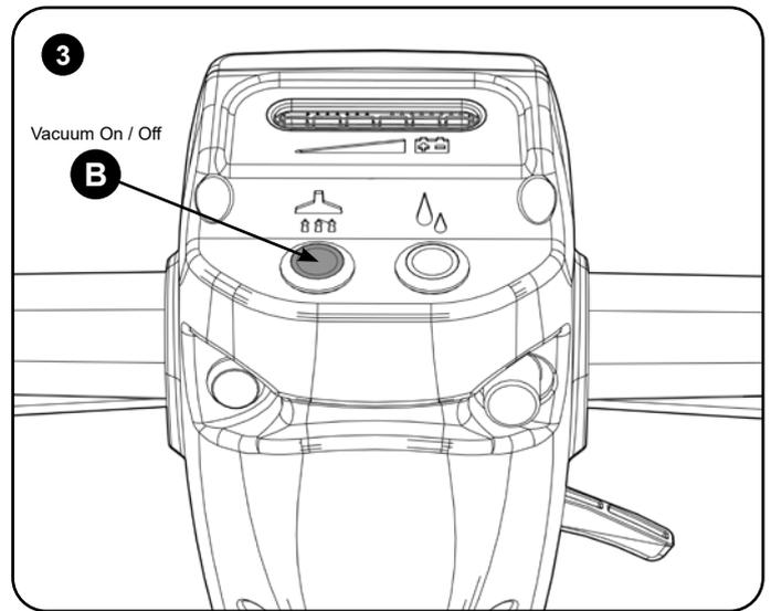
Press the vacuum on button, this lights up blue to indicate it is on and the vacuum starts. You are now ready to start cleaning.
