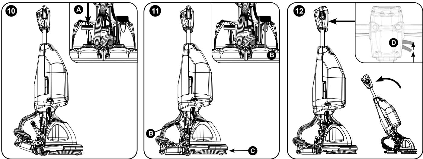
To lower the floor-tool, press down on the left foot pedal lever at the rear of the machine (10-A).
