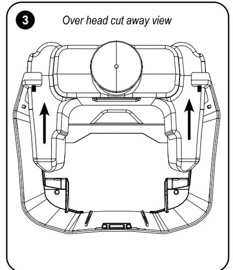
Remove the clean water tank from the main body of the tank holder.
