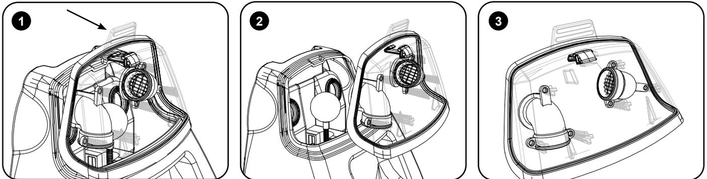
Using thumb and index finger grip the tab of the separator and pull forwards.
