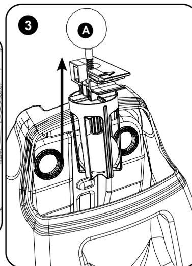
Lift the float valve from the tank, wash and inspect for damage.
