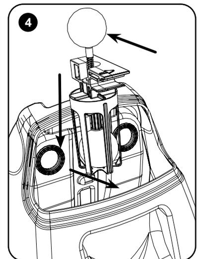
Place the float valve back down into the tank.
