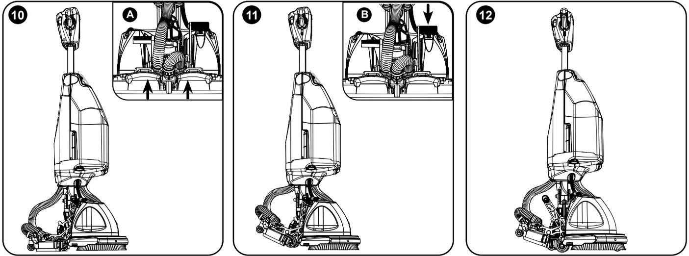
To raise the floor-tool use the toecap locations to the rear of the floor-tool and lift up (A). To raise the machine deck off the ground. Stand behind the machine, grip the handle. With your right foot push the right pedal down (B) while pulling the machine backwards until the storage wheels click into position and the front support wheel extends.
