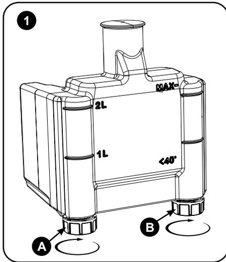
Make sure the clean water tank is empty. Unscrew the two clean water outlets, A and B.
