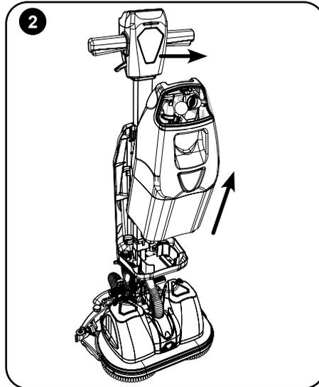
Lift and tilt the top of the tank assembly away from the handle as you remove. Place the tank assembly on a suitable surface in its upright/uppermost position.
