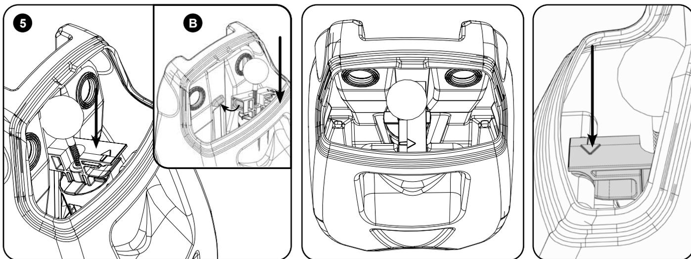
Tilt forwards at a slight angle making sure the protruding nub fits into the recess on the float valve (B).
