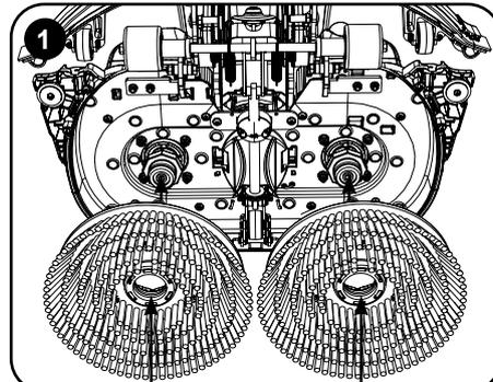
Push the brush / pad holder onto the brush motor mounts (1 & 2). *Note: Gloves are recommended to be worn whilst fitting and removing the brushes.*
