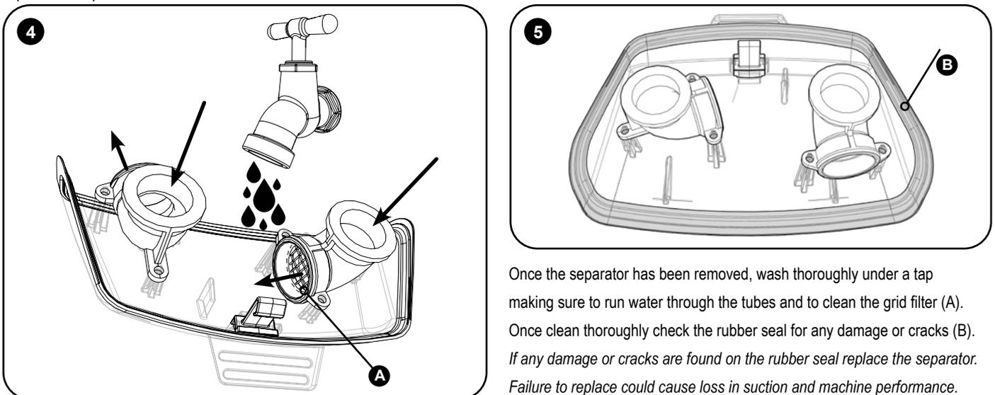
Once the separator has been removed, wash thoroughly under a tap making sure to run water through the tubes and to clean the grid filter (A). Once clean thoroughly check the rubber seal for any damage or cracks (B). If any damage or cracks are found on the rubber seal replace the separator. Failure to replace could cause loss in suction and machine performance.
