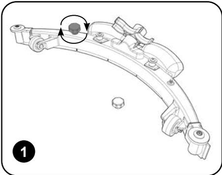
Unscrew the two knobs securing the blade holder (1).
