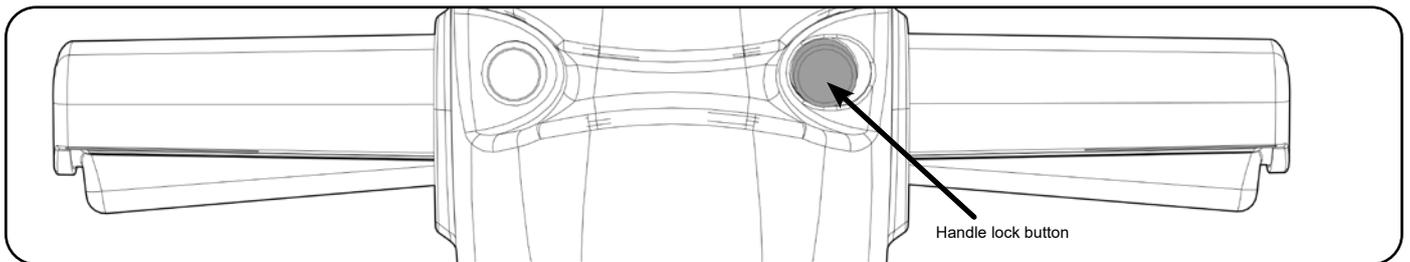
Make sure the handle is in the upright position and locked in place, push the handle lock button and locate handle in correct position.
