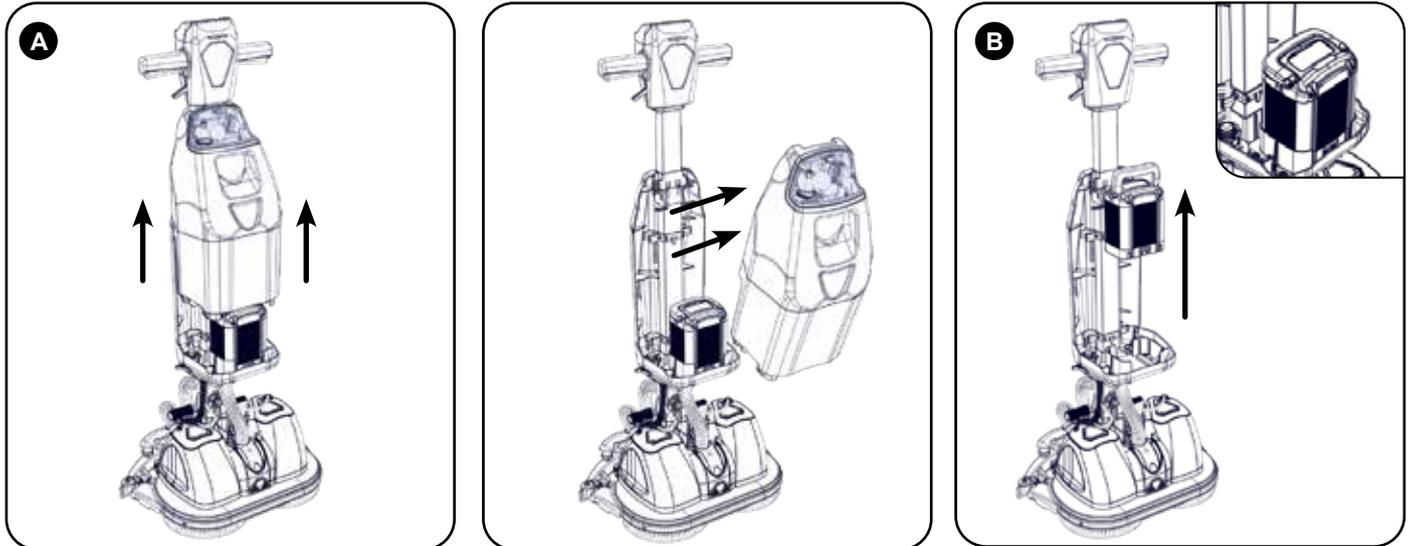
Remove the tank assembly from the front of the machine using the inset handle on the front of the tank assembly, lift the tank assembly straight up (A).
