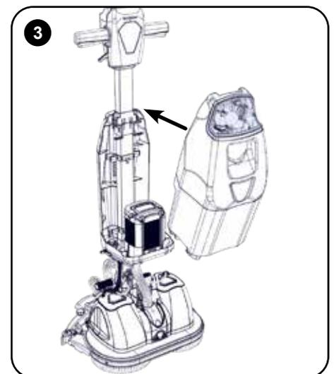
Lift the battery using the battery handle. Place the battery into the battery compartment ensuring it is securely in place and the orientation is correct (battery handle folds down towards the machine handle (A)).
