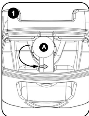
To remove the float valve twist the red retainer clip in the direction shown by the arrow on the retainer clip.
