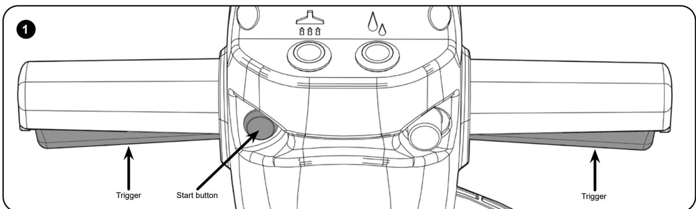
To start the machine pull one or both triggers in and press the start button with the deck down, this will start the brushes spinning and the battery power indicator will illuminate to show the power level.
