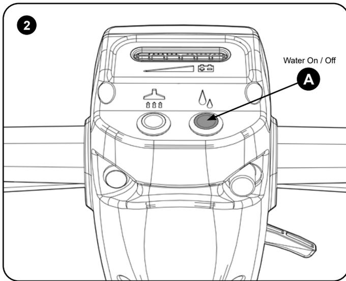
With either trigger pulled in press the water on button, this lights up blue to indicate it is on.
