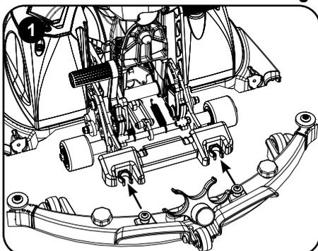
Push the floor tool carrier handle down and push the floor tool onto the retaining clips (1 & 2).
