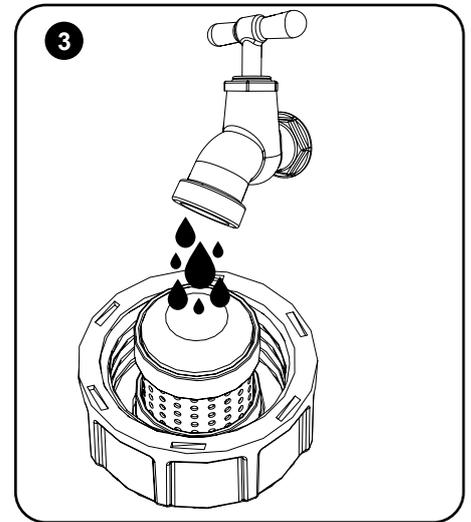
Wash the clean water outlets thoroughly under a tap, make sure the filter is clean with no blockages. Check for any damage (if any damage is found replace the clean water outlets).
