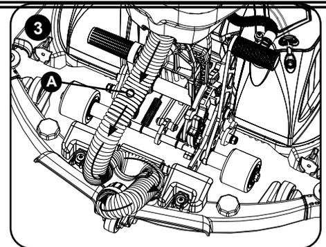
Take the hose and fit it into the hose retaining clips then push the open end securely over the centre fitting on the floor tool. Follow the arrows for the correct fit. Make sure part (A) of the hose stays loose and is not over stretched.
